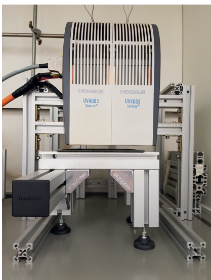
Fig. 3. Matrix removal in the repair area is carried out with the help of an UV LED lamp. Compared to conventional processes, the manual effort is highly reduced, which ensures higher reproducibility © ITM
